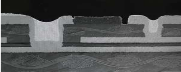
Cross section of PCB incorporating FaradFlex®
