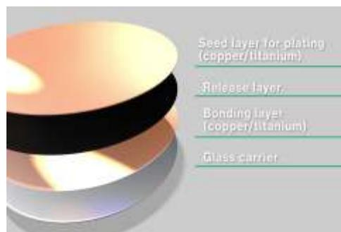
Functional layer thickness: 0.65 μm
