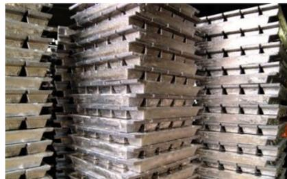
Unprocessed lead recovered by smelting recycled materials (example)
