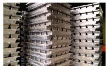
Unprocessed lead recovered by smelting recycled materials (example)
