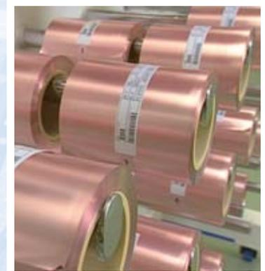
*Electrodeposited copper foil*
