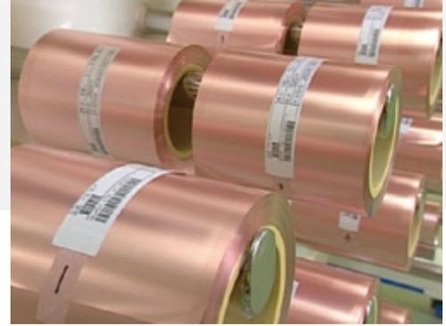
Electrodeposited copper foil
