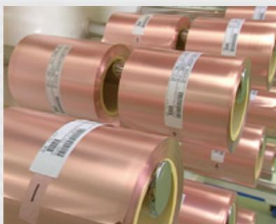
Electrodeposited copper foil
