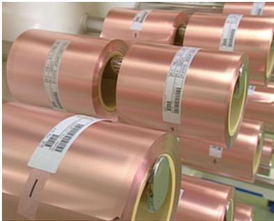
Electrodeposited copper foil
