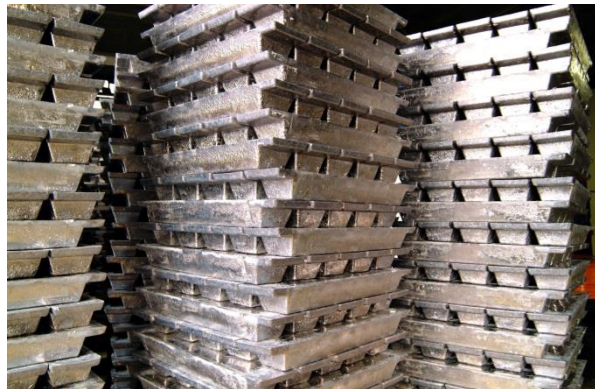
Lead ingots recovered by smelting recycled materials
