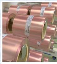
Electrodeposited copper foil
