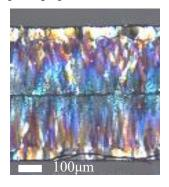
c-axis-oriented apatite-type lanthanum silicate solid electrolytes shows high oxide ion conductivity due to their orientation.
