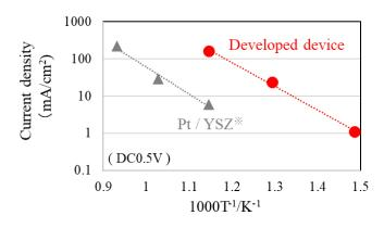
This developed device is capable of operation at lower temperatures (of approximately 200°C) than existing platinum electrode / yttria-stabilized zirconia (YSZ) devices.
